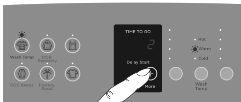
Fig.26 Adjusting the temperature setting, eg increasing the WARM wash temperature by 2°C
