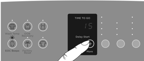
Fig.29 Modifying the number of beeps to signal the end of the cycle
